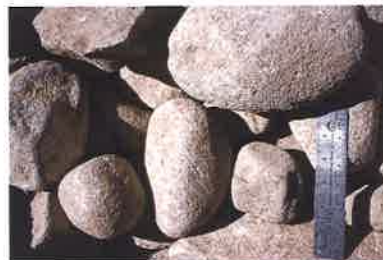
River Cobble 3-8 inch
